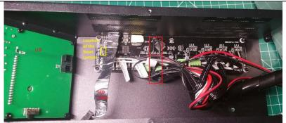
20. REASSEMBLE THE BOARD BY FOLLOWING STEPS 2-12 IN REVERSE ORDER. ENSURE THAT ALL CABLES ARE PROPERLY SEATED AND CONNECTED.
